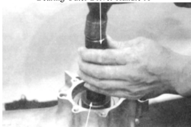
Bearing Outer Driver, 42x47mm Pilot, 20mm
