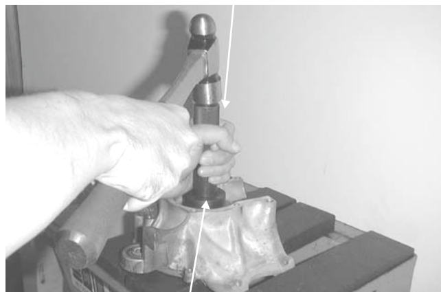
Bearing Outer Driver, 37x40mm Bearing Driver Pilot, 17mm
